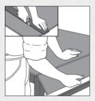
Power saw: Use a low-RPM portable saw with 89 mm (3-1/2 in.) carbide-tipped blade. To make cutouts for pipes and fixtures, use utility knife to cut through mesh on both sides of panel and punch out with a hammer from back side. Or, use an electric drill with a hole-saw bit.
