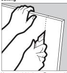
Line up straightedge or T-square with the marks and hold firmly against the face of the panel. Score through paper and lightly into the core. Use utility knife with sharp blade for scoring. To break the panel core, securely grasp
