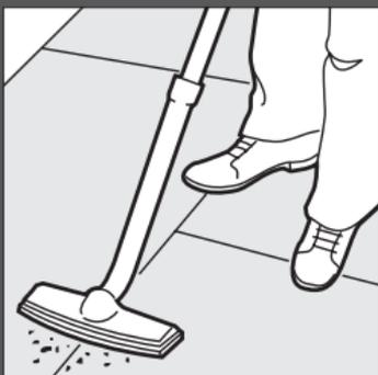
2. Substrate must be free of sealers, waxes, bond breakers, dust and dirt.
