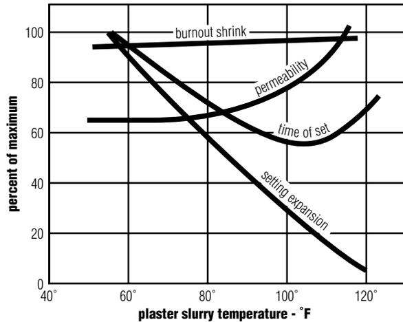
**Fig. 2**—Plaster slurry temperature effect on setting expansion, time of set, permeability and burnout shrink.
