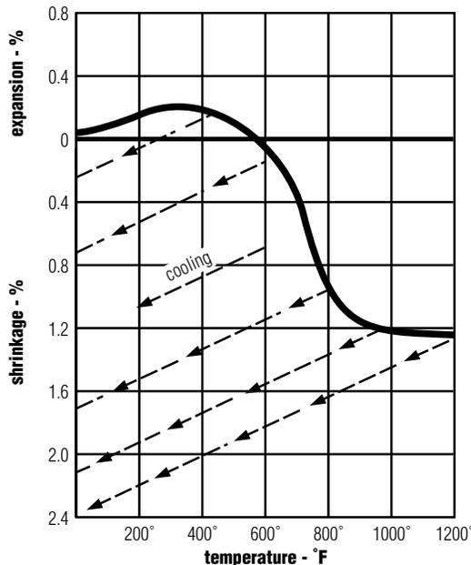
**Fig. 3**—Burnout temperature effect on burnout shrink.
