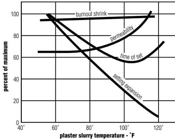
**Fig. 2**—Plaster slurry temperature effect on setting expansion, time of set, permeability and burnout shrink.
