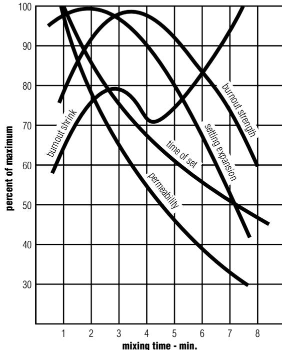
Fig. 1—Mixing time effect on time of set, permeability, setting expansion, burnout strength and burnout shrink.
