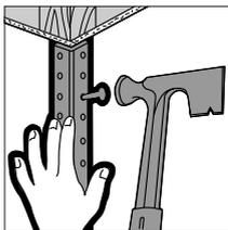
Install USG Metal Trim where gypsum panels butt window or concrete block. Nail trim every 9" through small holes in flange. Make sure that nails penetrate framing members.
