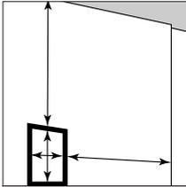
Mark the outline of the opening at the appropriate position on the gypsum panel. A template made from thin plywood is useful for repetitive cutouts.
