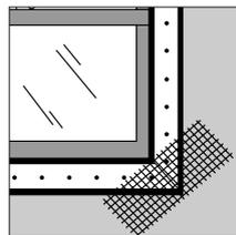
Crossstaping of mitered corners (diagonal application of tape, as shown above) is recommended. this prevents cracking that can be caused by movement of the two sections of bead.
