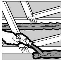
Select the proper adhesive for specific job requirements. Make sure that framing is clean, sound and free from oil, dirt or contamination. Apply adhesive and fasteners per instructions on adhesive cartridge. Do not use adhesive alone to secure panels unless specifically recommended by the adhesive manufacturer.
