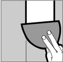
Apply SHEETROCK MH Brand Lightweight Setting-Type Joint Compound (TUF-SET Lite) or SHEETROCK Brand Lightweight Setting-Type Joint Compound (EASY SAND) to tapered joints using an 8"-10" knife the length of the joint.
