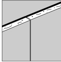
We recommend using a fiberglass mesh tape, such as TUF-TAPE, for finishing flat, tapered joints, and a paper tape, such as SHEETROCK Brand Joint Tape, for butt joints and corners.
