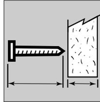
Drive nails in straight, not at an angle. Do not overdrive or countersink nails. This results in breaking the face paper or fracturing the gypsum core. If a nail happens to go in crooked, hold the panel tight against the framing and drive a second nail in about 2" from the nail that punctured the paper. Then drive the first nail in below the surface of the board.
