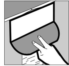
The tapered joint should then be feathered, with the compound spread out very thin at the edges. To feather, press down on the edge of the knife that is furthest from the joint, and lift the other edge very slightly.
