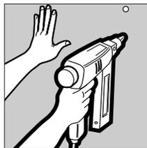
Seat nail so head is in a shallow dimple (1/32") in the face of the drywall.
