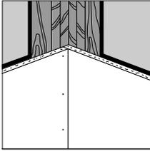
To join panels at an outside corner, lap the end of the second board over the end of the first, and fasten both panel ends to their common stud.
