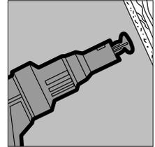
Use an electric or pneumatic screwgun equipped with an adjustable screw depth control head and Phillips bit. Drive screws in straight, leaving the screwhead slightly (1/32") below the face of the gypsum board. Be careful not to overdrive screws. Breaking the face paper greatly lessens the holding power of the screw.
