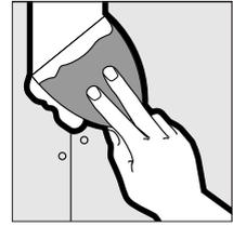
Center and lightly press tape into wet joint compound with fingers. Draw 6" knife firmly along joint to tightly embed tape. Be sure there is sufficient joint compound under tape to prevent blistering of the tape.
