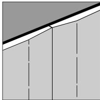
Butt joints occur where the cut edges of two panels butt together. Because there are no tapers at butt joints, the tape and compound will automatically lie on top of the surface of the board. This means that butt joints are always naturally crowned, and will require a slightly different finishing procedure.
