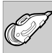
The banjo has a hinged side panel for hand-loading compound into the tool, and an adjusting slide to control the amount of compound dispensed onto the tape.
