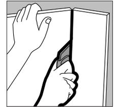
After cutting the panel, smooth the cut edge with a rasp. Be sure to keep edge as square as possible. Always wear a dust mask when sanding or rasping.
