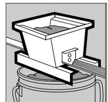
Always be sure to place the hopper so that the gate on the exit side (where the bead, with compound applied, will leave the hopper) matches the profile of the bead.
