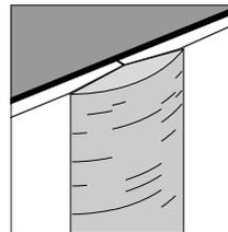
To prevent starved and crowned joints, two different techniques of applying joint compound are used. These are known as "centering" and "splitting." You should center a tapered joint by first running the knife down the center, then up one side, then down the other, then down the middle again. This will ensure that the depression created by the tapers will be filled.
