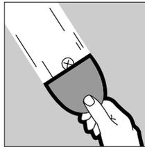
Remove any loose paper, and cut out any soft spots or bulges in the board.
