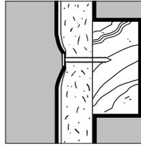
For 1/4", 3/8", and 1/2" thick panels, use 1-1/4" annular ring drywall nails. For 5/8" panels, use 1-3/8" annular ring drywall nails.
