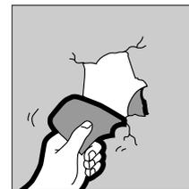
Apply a skim coat of joint compound with a joint-finishing knife to damaged area and feather to get a smooth finish. Let dry and apply second coat if necessary. Sand and prime when dry.
