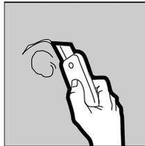
Butt joints, where cut board edges meet, should be cut with a "V" groove to remove fuzzed paper.
