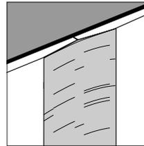
Butt joints, on the other hand, are naturally crowned, because the tape and compound have to be placed above the surface of the board. Excess compound will result in a crowned joint.
