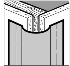
If regular right-angle bead is to be used for an outside corner, the boards should overlap as usual.
