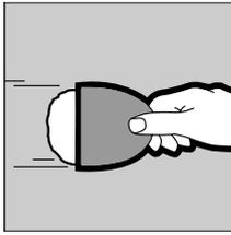
Then raise the knife blade to a more upright position and scrape off excess with a second stroke at a right angle to the first stroke. Compound should be level with panel surface.
