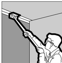
Attach the corner finisher to the angle applicator, then fill the angle applicator using a hand pump attached to a box-filler adapter. Keeping the corner finisher head over the edge of the joint compound bucket, pump until the applicator is full.
