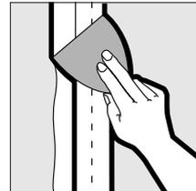
While embedding the tape, remove excess joint compound from edge and apply as a thin coat over the tape.
