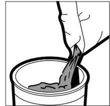
Mix thoroughly by hand or using a power mixer, as indicated on packaging. If you are power-mixing, use a mixing paddle designed for joint treatment and textures, and use a drill with a maximum speed of 450 rpm.
