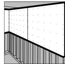
Apply lower row of panels so that tapered edges meet with those of top row. Vertical joints should be staggered. Avoid vertical joints directly above or below the corner of a window, door, or other opening for best decorating results.
