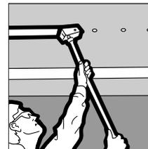
The nail spotter can be filled with compound using a pump and adapter.
