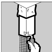
**CAUTION:** It is difficult to fold fiberglass tape to achieve a straight interior corner. In addition, the use of fiberglass tape can cause a buildup of compound in the corner that will result in cracking later on. Therefore, the use of paper tape in corners is recommended. As an alternative, paper-faced metal bead can also be used for corner reinforcement.
