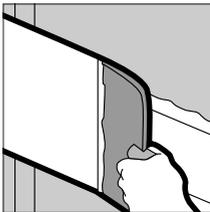
Apply pressure to knife edge farthest from the joint and lift the other edge just slightly above surface. Draw knife down joint. Repeat for opposite edge. This technique is called feathering. Joint compound should extend beyond first coat for a total width of 7" or 8". Apply a 7"-8" coat of joint compound to each side of butt joints and feather. Compound should extend beyond first coat for a total width of 14"-16".
