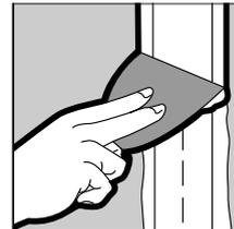
To finish tapered joints, follow same procedure. Tape should overlap tape applied to butt joints.
