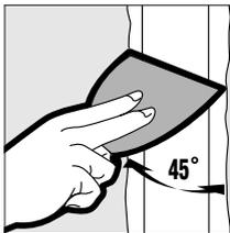
To apply joint compound neatly, dip the knife and strike excess compound from the sides of the knife to keep the material centered.
