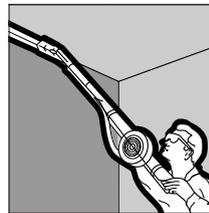
Avoid twisting the taping tool. As soon as possible, begin operating the tool at a 45° angle to the joint. This will help prevent tape "creeping."
