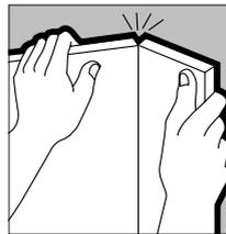
Use utility knife with sharp blade for scoring. Complete cutting by running knife through back paper for the length of the panel and snapping back to face.
