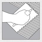
Working a small area at a time, press tile into place with a slight twisting motion to seat properly. Prevent adhesive buildup on tile edge and in grout space. If adhesive squeezes from under tile, remove excess before it dries.
