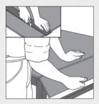
Power saw: Use a low-RPM portable saw with 3-1/2 in. (89 mm) carbide-tipped blade. To make cutouts for pipes and fixtures, use utility knife to cut through mesh on both sides of panel and punch out with a hammer from back side. Or, use an electric drill with a hole-saw bit.
