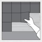
Keep tiles and joints straight and uniform. Use tile spacers if desired.
