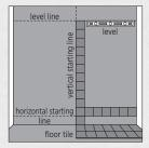
On bathroom floors, start by placing full tiles in front of bathtub or shower and along the adjoining wall to avoid cut tiles in this highly visible area.
