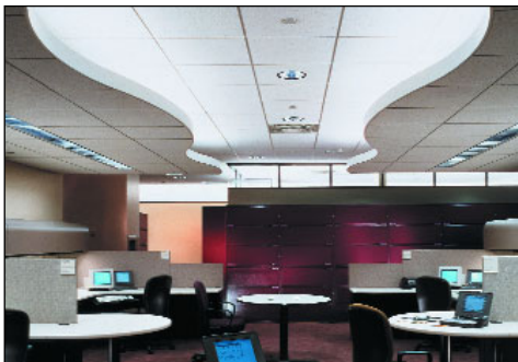
Suspension trim enables the creation of free-form island ceilings and fascia.
