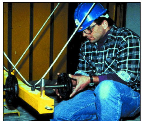
A weighted swinging ram replicates “real-world” conditions by simulating the direct-concentrated impact of a tool or hard object against a wall system.
