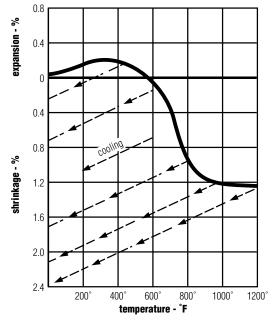
Fig. 3—Burnout temperature effect on burnout shrink.
