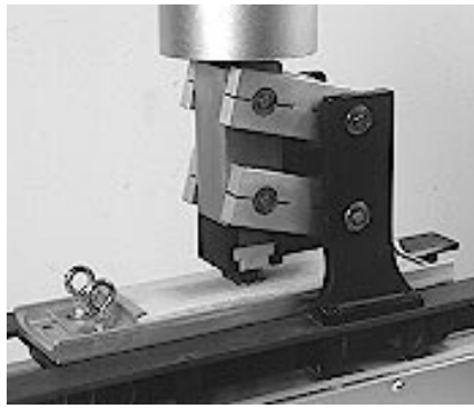
Fig. 2. Abrasion damage is measured using testing apparatus with weighted steel brush.
