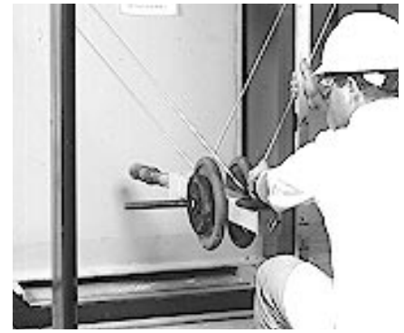
Fig. 3. Impact damage is measured using testing apparatus to approximate sledge hammer impact.
