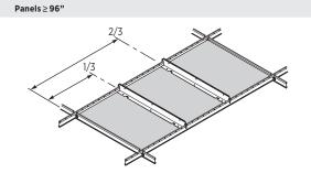
If opening is  $\geq 96$ " then two stabilizer bars are required at the 1/3 and 2/3 points.
