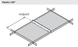
If opening is  $\geq$  60" then one stabilizer bar is required at midpoint.
