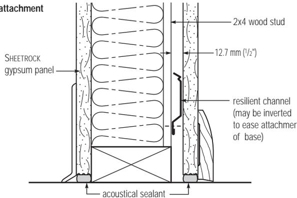
Ceiling/floor attachment/SHEETROCK gypsum panel, FIRECODE C Core panel
