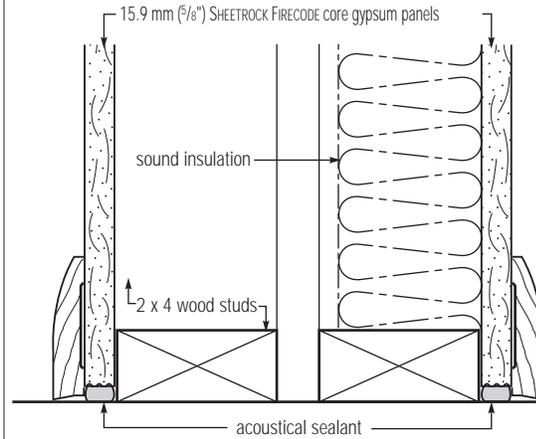
Ceiling/floor attachment — SHEETROCK gypsum panel
