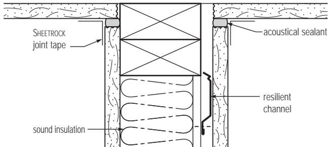
Ceiling/floor attachment/SHEETROCK gypsum panel, FIRECODE C Core panel
