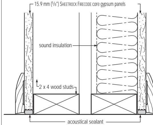
Ceiling/floor attachment — SHEETROCK gypsum panel
