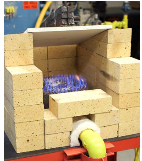
Figure 3: 13" x 13" sample of CGC Sheetrock® Firecode C Gypsum Panel with a 16 lb. 13 oz. weight located in the centre to dramatize the failure point.
