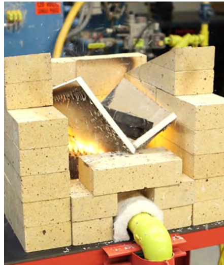
Figure 4: After 57 minutes, the CGC Sheetrock® Firecode X Gypsum Panel collapsed due to the thermal exposure and the superimposed load.
