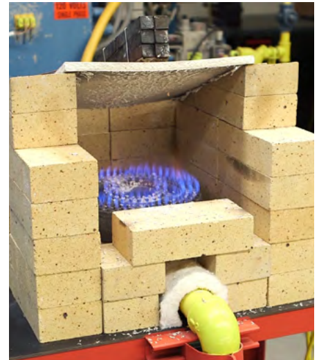
Figure 5: After two hours two minutes, the CGC Sheetrock® Firecode C Gypsum Panel showed no signs of failure and the test was terminated. The Type C panel resisted failure for over twice as long as the Type X panel.
