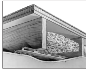
Wood-frame—with resilient attachment and THERMAFIBER SAFB.
