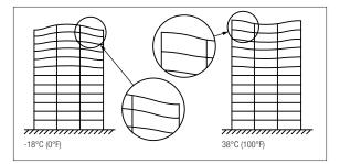
contract in length. The amount of expansion or contraction of the exposed columns depends on the temperature difference and several other factors. (Structural movement caused by thermal differentials accumulates to the upper floors.) However, the stiffness of the structure resists the movement and usually full unrestrained expansion is not reached. A gypsum board wall 30 m (100') long will expand 14 mm (0.54') when the temperature rises 28C° (50F°).
