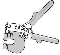
**Pop Rivet Tool** Plier-type tool used to flare and secure pop rivets through prepared holes. Especially useful for securing wall angle corners or tee joints in suspended acoustical ceiling applications.
