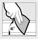
To apply drywall compound neatly, dip the knife sideways into the pan so you load only half the width of the blade.
