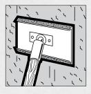
Before applying the final coat, check to see if tapered joints are level with surface. Hold the 250 mm (10 in.) blade across the joint, straight out from the wall. If the blade can be rocked across the joint, the joint is crowned. It must be hidden by feathering the final coat out as far as possible.
