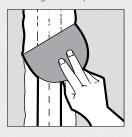
While embedding the tape, remove excess drywall compound from edge and apply as a thin coat over the tape.
