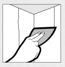
Fold tape along center crease and lightly press into position with your fingers.
