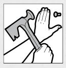
Seat nail so head is in a shallow dimple formed by last blow of drywall hammer.
