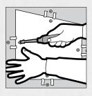
d. Remove tabs from each drywall repair clip. Apply compound and tape to all four section sides. Do not overlap tape. Apply second and third coats of drywall compound, allowing each coat to harden before applying next coat and feathering out from previous coats. Sand and prime when dry.
