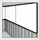
Apply lower row of panels so tapered edges meet with those of top row. Vertical joints should be staggered. Avoid vertical joints directly above or below a window, door or other opening for best decorating results.
