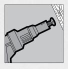
Use an electric screwgun equipped with an adjustable screw depth control head and Phillips bit.
