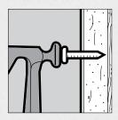
Double-nailing reduces the likelihood of nail pops. It is highly recommended for ceilings. Drive first nails 300 mm (12 in.) o.c. along framing in the field of the board and second nails about 50 mm (2 in.) from the first. Fasten the perimeter 180 mm (7 in.) o.c. for ceilings and 200 mm (8 in.) o.c. for walls.
