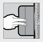
When applying earlier coats, 18 SANDING minor depressions and grooves were not a problem. However, do not leave any during the application of this final coat or they will mar the finished surface.
