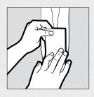
d. Apply compound over tape with knife. Let harden and apply second coat of compound if necessary. Sand and prime when dry.
