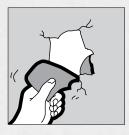
b. Apply a skim coat of drywall compound with a drywall finishing knife to damaged area and feather to get a smooth finish. Let dry and apply second coat if necessary. Sand and prime when dry.
