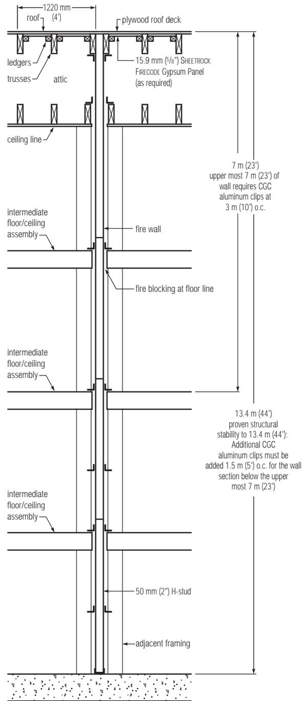
**Typical firewall roof parapets (height as required by code)**
