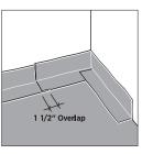
4. For inside corners, provide a relief cut, but place adhesive where the membrane folds over itself to ensure a water-durable connection. Overlap butt joints by 1-1/2" and use the mastic to ensure a water-durable connection. Apply adhesive to the vertical and horizontal legs of the butt joint. Work the material carefully into position and smooth out, using the flat edge of the trowel.
