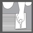
Install membrane with cementitious side out. Embed into adhesive, using the flat edge of the trowel or with a nonsegmented hand roller. Start in the center of the sheet and work out toward the edges, removing all air bubbles. Overlap each row 2", making sure that a sufficient amount of adhesive is applied to the joint area.
