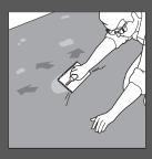
Areas unable to receive vertical flashing, such as pipe penetrations and bathroom tubs, should be sealed using a good quality silicone sealant. Run a continuous bead and tool the material to provide continuity to the membrane.
