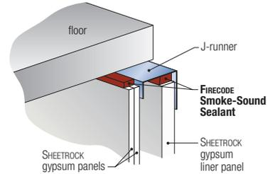
FIRECODE Smoke-Sound Sealant is also rated for joints in shaft wall assemblies and can be used with most liner panel systems, including, but not limited to, U415.
