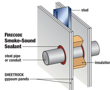
FIRECODE Smoke-Sound Sealant is classified for use in through-penetration fire stop systems C-AJ-1020 and W-L-1064 and complies with IBC requirements for smoke barriers.
