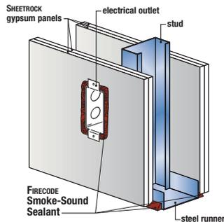
Sound-seal partitions at gaps, cutouts and dissimilar materials on both sides to maximize STC/MTC of an assembly with FIRECODE Smoke-Sound Sealant.
