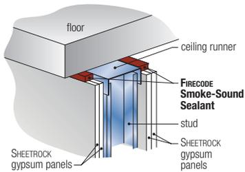
A UL-classified fire and smoke caulk, FIRECODE Smoke-Sound Sealant is ideal for head-of-wall and bottom-of-wall systems in fire-rated partitions and smoke barriers.
