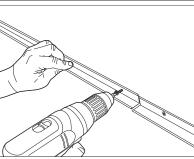
With no support between lengths of trim, traditional wall angle is more difficult to install. Butt-cut wall angle is also subject to misalignment of trim faces and gaps at joints.
