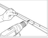
Overlap detail sits on adjacent trim, providing extra support for quicker, easier installation. The overlap ensures that trim faces are level, and it eliminates the unsightly gap created by traditional butt joints.
