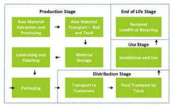
panels are packaged for shipment. Panel trim and panels that are chipped or broken during manufacturing are sent to landfill. The Cloquet plant produces its own paint coatings and the primary ingredients for these coatings are also included in the analysis.
