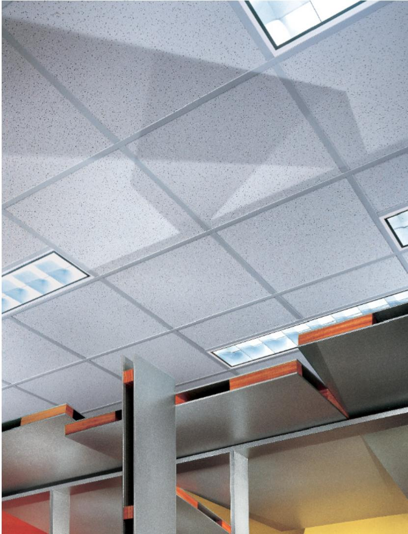
***RADAR FIRECODE, RADAR CLIMAPLUS FIRECODE, RADAR CLIMAPLUS High-NRC/High-CAC FIRECODE acoustical ceiling panels are economical, wet felted mineral fiber and medium-textured panels that feature a non-directional pattern and offer FIRECODE and optional anti-sag performance. They install quickly and easily and are classified as low-emitting ceiling panels for offices, schools, corridors and retail stores.***
