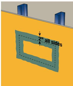
**D:** Apply Dymonic 100 (green) sealant at 40 mil thickness over the entire surface of the repair patch and extending 2" beyond the gaps on all sides.
