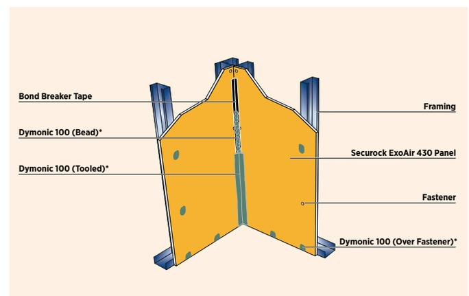
*\*Spectrem 1 is an alternative to Dymonic 100, but cannot be used with an adhesively-applied cladding.*
