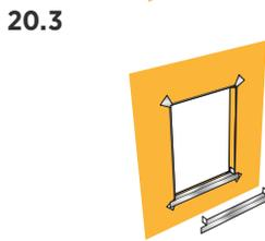
**Sill:** Cut a strip of ExoAir 110AT 6” longer than the length of the sill’s opening. For example, a 36” sill will require a 42” strip of ExoAir 110AT. Fold the strip in half lengthwise. Make a 3” cut along the fold at each end so that you have two flaps. This will allow the sheet to be easily positioned into the rough opening and on to the exterior face of the panel.
