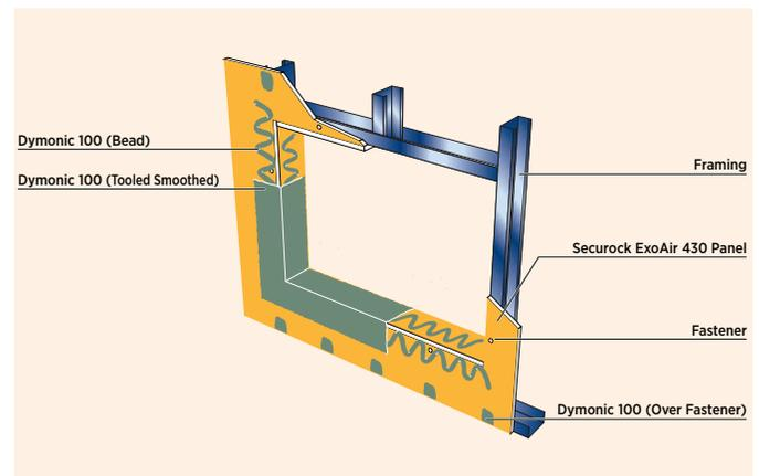
**17.3** Tool Dymonic 100 (green) sealant on the face of the panel toward the rough opening ensuring the exposed core is covered with no holes or gaps. Feather sealant out onto the panel. Tool Dymonic 100 (green) sealant in the rough opening toward the face of the panel ensuring the exposed core is covered with no holes or gaps. Measure sealant to ensure that at least 40 wet mils have been applied; if not reapply Dymonic 100 (green) sealant.
