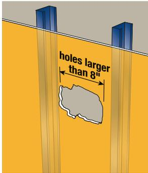
**A:** For openings or gaps larger than 8" in any direction, the panel shall be repaired as follows.
