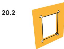
Cut ExoAir 110AT into four “bow tie” shapes. Length 6”, top / bottom width 3”, center 1”. Remove backing and center the 1” section of the bow tie over face of joint. Press half onto the face of the panel and half into the rough opening. Mechanically roll to smooth out any fish mouths or air pockets in the membrane. Complete all four corners before applying flashing to the rough opening.
