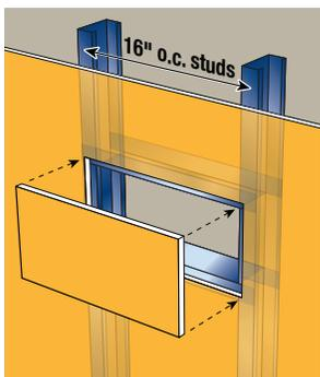
**B:** Cut the panel back to the framing on parallel sides. Cut a piece of Securock ExoAir 430 Panel to tightly fit into the opening and secure to framing with screws. Gaps between boards shall not exceed 1/8". Ensure all surfaces are clean, dry and free of dust or debris.
