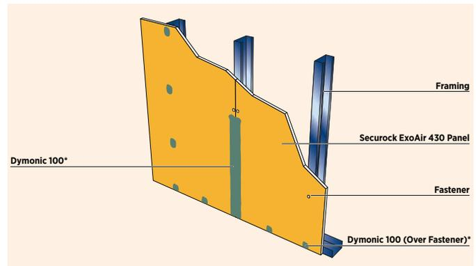
*\*Spectrem 1 is an alternative to Dymonic 100, but cannot be used with an adhesively-applied cladding.*
