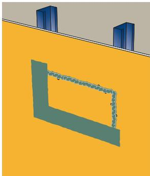
**C:** Caulk all gaps with Dymonic 100 (green) sealant, completely filling the gaps and tool smooth.
