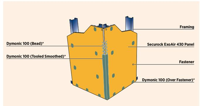
*\*Spectrem 1 is an alternative to Dymonic 100, but cannot be used with an adhesively-applied cladding.*
