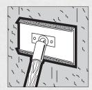
Before applying the final coat, check to see if tapered joints are level with surface. Hold the 10" blade across the joint, straight out from the wall. If the blade can be rocked across the joint, the joint is crowned. It must be hidden by feathering the final coat out as far as possible.
