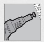
Use an electric screwgun equipped with an adjustable screw depth control head and Phillips bit. If an electric drill is used, be careful not to overdrive screws.
