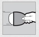
Then raise the knife blade to a more upright position and scrape off excess with a second stroke at a right angle to the first stroke. Compound should be level with panel surface.
