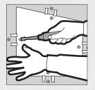
d. Remove tabs from each drywall repair clip. Apply compound and tape to all four section sides. Do not overlap tape. Apply second and third coats of joint compound, allowing each coat to harden before applying next coat and feathering out from previous coats. Sand and prime when dry.
