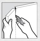
After cutting the panel, smooth the cut edge with a drywall rasp or sandpaper wrapped around a block of wood such as a piece of 2" x 4" lumber. Be sure to keep edge as square as possible. Always wear a dust mask when sanding.
