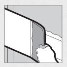
Apply pressure to knife edge farthest from the joint and lift the other edge just slightly above surface. Draw knife down joint. Repeat for opposite edge. This technique is called feathering. Joint compound should extend beyond first coat for a total width of 7" or 8".
