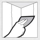
Fold tape along center crease and lightly press into position with your fingers.
