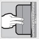
When applying earlier coats, 20 SANDING minor depressions and grooves were not a problem. However, do not leave any during the application of this final coat or they will mar the finished surface.
