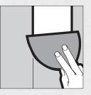
Apply joint compound to tapered joints using an 8" knife the length of the joint.
