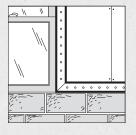
Install USG Metal Trim where gypsum panels butt windows or concrete block. Nail trim every 9" through small holes in flange. Make sure that nails penetrate framing members.
