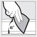
To apply joint compound neatly, dip the knife sideways into the pan so you load only half the width of the blade.
