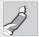
c. Crisscross two or three strips of joint tape over opening and embed tape in joint compound. Let harden.
