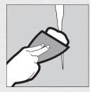
c. Embed tape in compound to bridge crack. Draw knife firmly over crack to tightly embed tape. Let compound harden.
