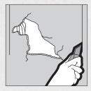
b. Slip drywall repair clips onto the edge of the damaged wall. Position screws about 3/4" in from the edge and centered between the tabs. This will line up the screws with perforations in the clips. Screw through wall into each drywall repair clip.
