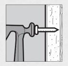
Double-nailing reduces the likelihood of nail pops. It is highly recommended for ceilings. Drive first nails 12" o.c. along framing in the field of the board and second nails about 2" from the first. Fasten the perimeter 7" o.c. for ceilings and 8" o.c. for walls.
