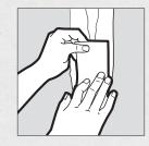
d. Apply compound over tape with knife. Let harden and apply second coat of compound if necessary. Sand and prime when dry.
