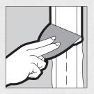
To reinforce tapered joints, follow same procedure. Tape should overlap tape applied to butt joints.
