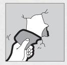
b. Apply a skim coat of joint compound with a jointfinishing knife to damaged area and feather to get a smooth finish. Let dry and apply second coat if necessary. Sand and prime when dry.
