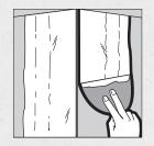
Using a 6" taping knife for outside corners (4" for inside corners), apply another coat of joint compound (USG Sheetrock\* Brand Easy Sand<sup>M</sup>, Topping, All Purpose, or Lightweight All Purpose). Keep this coat as smooth as possible. Feather out 5" to 6" (125 to 150 mm) from the nose of the trim on each side for outside corners (1" or 25 mm past previous coat for inside corners). Let dry. Sand sides lightly where needed.
