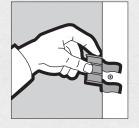
c. Measure and cut new drywall panel section to fit damaged area. Screw through new drywall into each drywall repair clip. Screw into drywall, positioning screw opposite screw holding clip and about 3/4" from edge.
