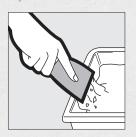
While embedding tape, draw the knife slowly along the length of the tape to provide an even distribution of joint compound. Don't worry about a few grooves or streaks in the joint compound. They will be covered over in the subsequent coats.
