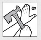
Seat nail so head is in a shallow dimple formed by last blow of drywall hammer.
