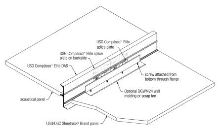
ISO Exploded - DAS Drywall Lower to Acoustical Upper Assembly Splice
