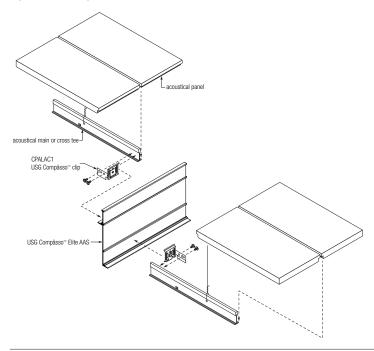
Exploded - USG Compässo™ Elite Drywall to Acoustical Transition
