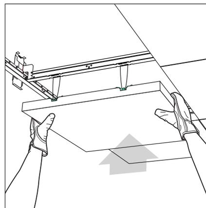
**Step 10: Install the USG Compässo® Trim onto the trim clips.**
