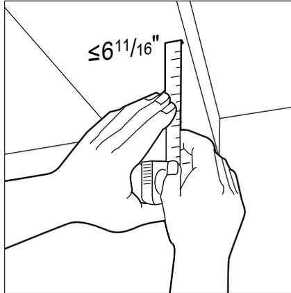
**Step 2a: Mark the ceiling height at the perimeter.**
