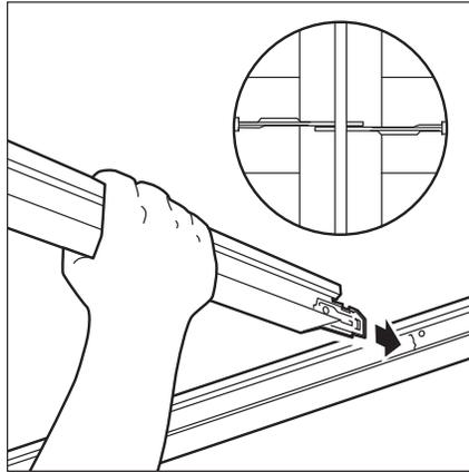
**Step 6: Install the USG Compasso® Trim clips onto the perimeter tees.**
