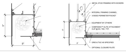
At each end of the pocket determine if the system will continue with another section, turn 90-degrees or terminate with an end cap.
