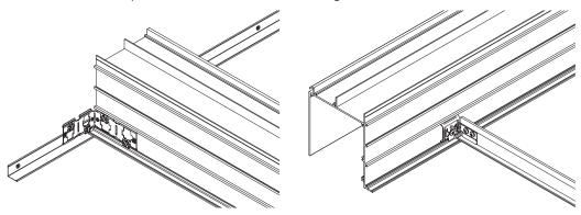
STEP 3 Connecting the pocket to the acoustical ceiling with a standard Compässo™ Elite attachment clip (279543). Mounting the clip along the splice channel at the desired take off point for the grid system.
