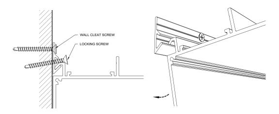
Choose a ceiling height and determine the mounting strategy. USG offers three (3) mounting options with these systems; the wall cleat/extrusion hook mounting, hanger wire mounting or metal framing member installation.
