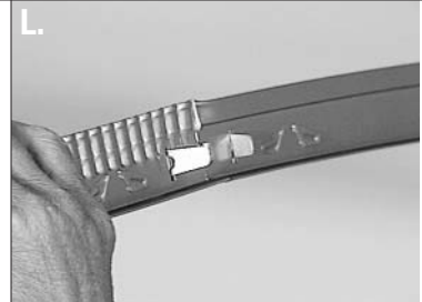
To connect Main Tees, use a Main Tee Splice. Insert the splice tabs into the slots at the ends of the adjoining Main Tees. Then, partially bend the tabs inward.
