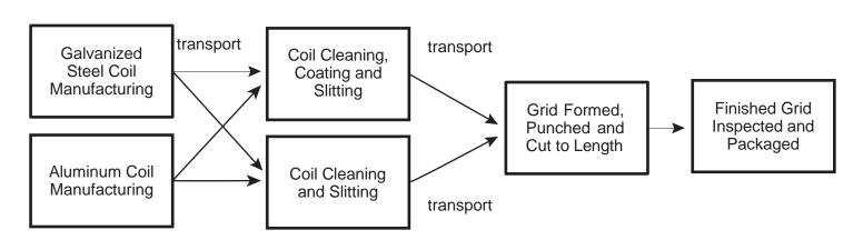
During the grid production process, a piece of galvanized steel coil (destined to be the body) and a second piece of coated galvanized steel coil or coated aluminum coil (destined to be the cap) are combined into the proper configuration using a series of driven dies. A clip is attached to both ends of the main tee and cross tee members allowing for connection of the various pieces.
