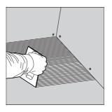
**5.** Apply additional mortar, combing it in a single direction using a 1/4 in. x 1/4 in. square-notched trowel.
