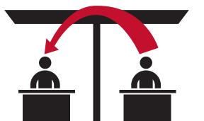
CAC: Applies to the sound attenuation of acoustical ceilings with a shared plenum above horizontally adjacent spaces.
