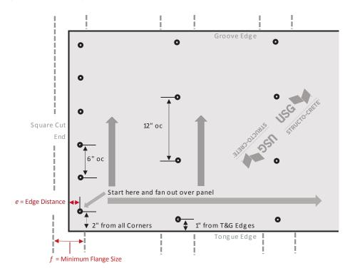
**Fastener Quantities:** This is intended to be a starting point for fastener estimating only. USG recommends that a calculation be made for each project layout to determine the appropriate number of fasteners required and that an excess of at least 10% be added to the calculated quantity for the project.
