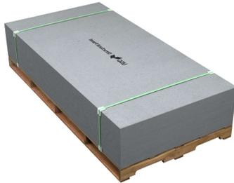
USG Structural Panel Concrete Subfloor, also known as USG Structo-Crete™ Panel, is a mechanically attached concrete subfloor that can be combined with other noncombustible materials to create 1-, 2- and 3-hour fire-rated floor-ceiling assemblies.
