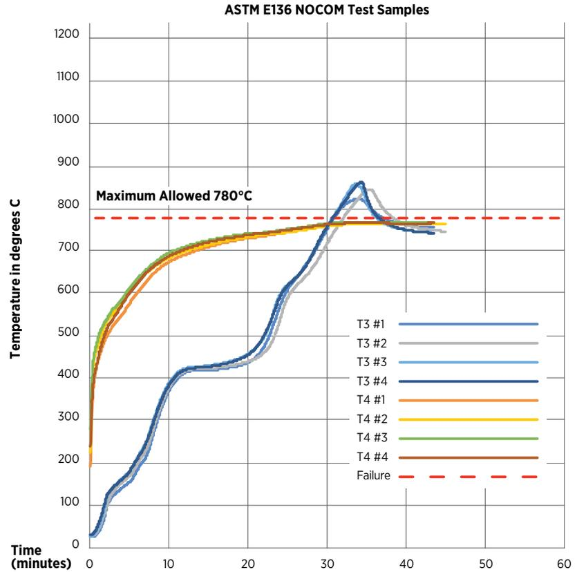
Figure 3 - NOCOM Time/Temperature Curves
