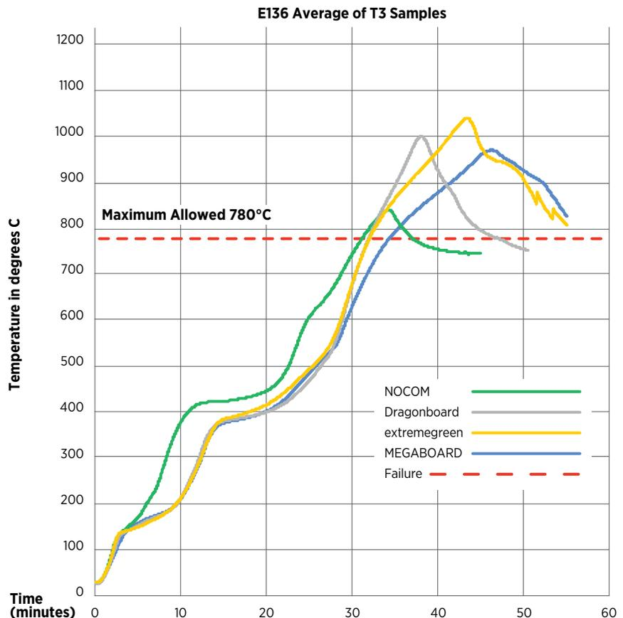
Figure 9 - ASTM E136 T3 Sensors Average Time/Temperature Curve
