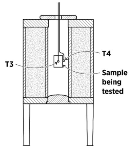
**Figure 1 - Vertical Tube Furnace Locating T3 & T4 Sensors**
